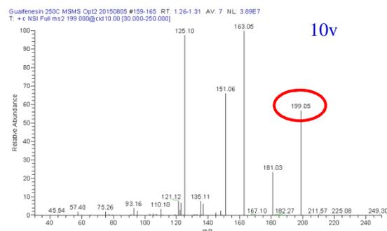
Fig.1: DART-MS-MS spectra of Guaifenesin standard (199.0 m/z) at 10v
