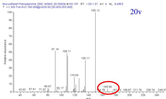
Fig.5: DART-MS-MS spectrum of Phenylephrine in Mucus Relief at 20v
