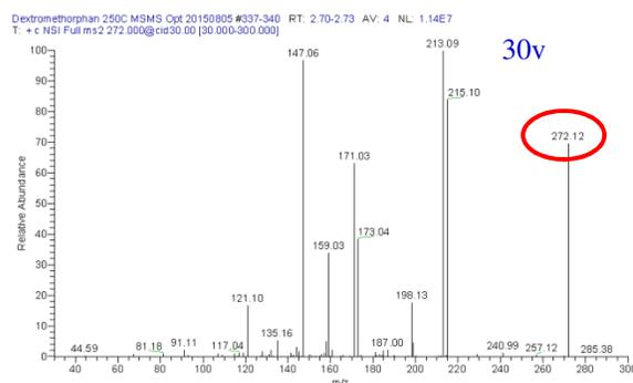
Fig.3: DART-MS-MS spectra of Dextromethorphan standard (272.0 m/z) at 30v
