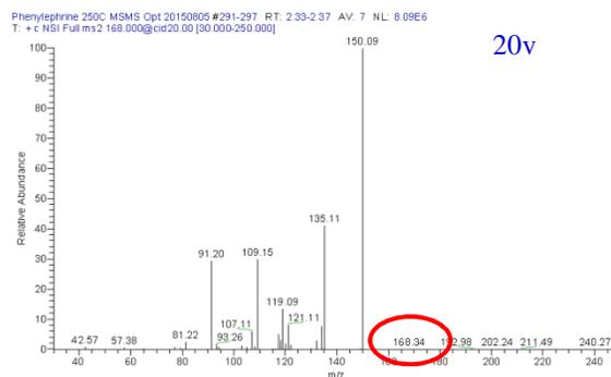
Fig.2: DART-MS-MS spectra of Phenylephrine standard (168.0 m/z) at 20v
