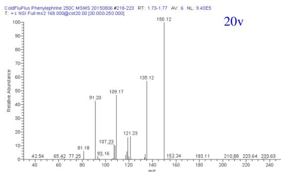
Fig.6: DART-MS-MS spectrum of Phenylephrine in Cold & Flu at 20v
