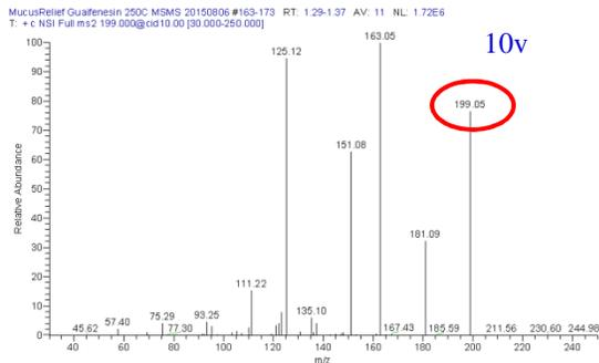
Fig.4: DART-MS-MS spectrum of Guaifenesin in Mucus Relief at 10v
