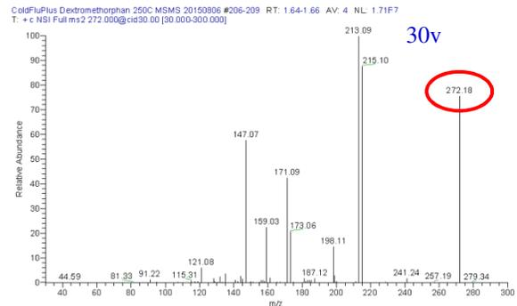
Fig.7: DART-MS-MS spectrum of Dextromethorphan in Cold & Flu at 30v
