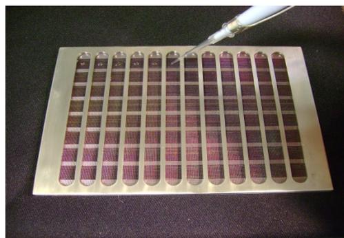
Image 2 – Pipetting onto an X-Z mesh holder
