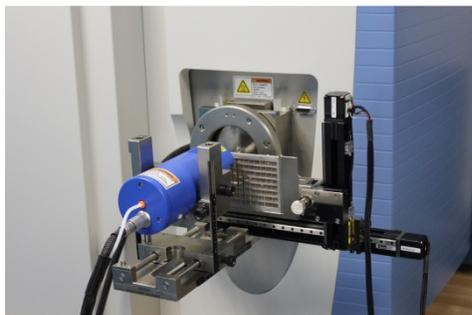
Image 1 – The DART XZ-Scanner coupled to a MS
